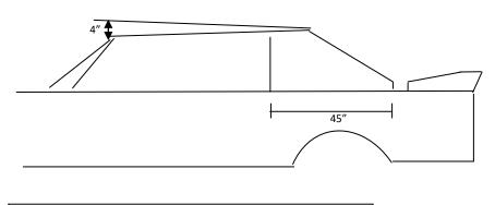
Sail panels and spoiler with supports to resemble this style. Sail panels cannot tie spoiler side supports.
